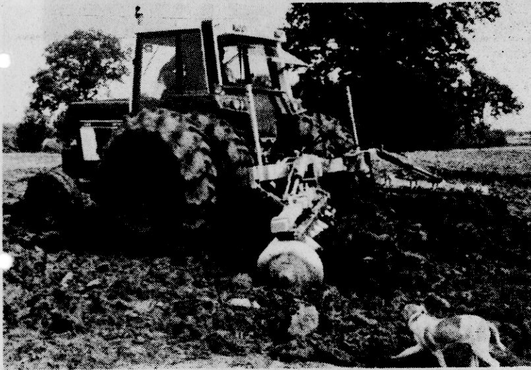
Ole Spot inspects the terrace plow which was demonstrated on the Hughes Brothers farm near Jumpertown this past spring. Building terraces with the new disk type terracing plow is much faster than other methods of terrace construction. Prentiss County farmers installed over 27,000 feet of terraces this past year. Due to terrace installation and other conservation practices such as minimum tillage, delayed seedbed preparation and contour farming, over 3,700 acres of cropland was adequately protected from soil erosion. Prentiss County farmers and landowners are encouraged to use terrace systems when needed to reduce soil erosion.
